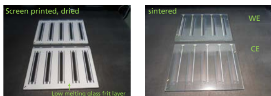
Figure 5: Photos of the screen-printed in-situ PSC test cells during manufacturing; The layer sequence and the approximate layer thickness after sintering have been the following: Working electrode (WE): glass - TCO – 10 nm TiO 2 n-selective layer – 400 nm nano-TiO 2 mesoscopic layer – 300 nm porous ZrO 2 isolation layer – 10 μm porous graphite layer composition. Counter electrode side (CE): glass -TCO – 10 μm porous graphite layer composition. During the sintering the glass frit layer has been molten (glazed) as can be seen by the transparent appearance (photo on the right side).
